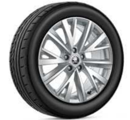
Gigaro light-alloy wheel 7.5J × 18" ET40 for 235/55 R18 57H 071 498 8Z8 | silver metallic, brushed
